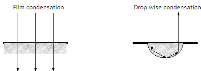
Figure 2-37. Effect of condensation on light transmission
