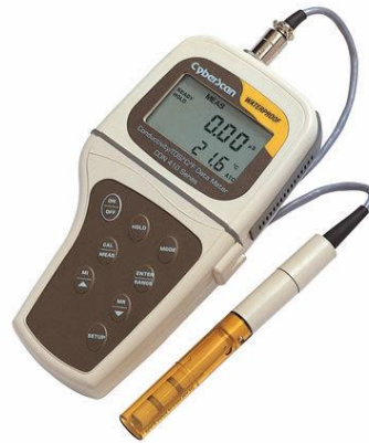
Figure 11-18. Handheld conductivity meter ( http://www.eutechinst.com )
