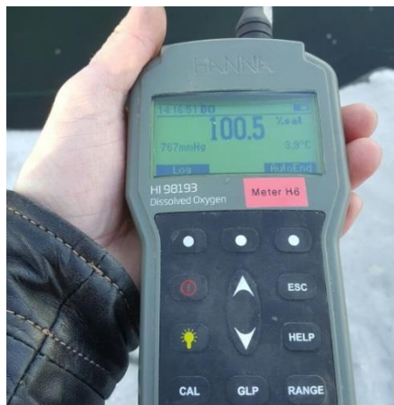
Figure 6-20. Measurement of the dissolved oxygen of the water storage of Proeftuin Zwaagdijk (The Netherlands) where a floating Airlift is installed
