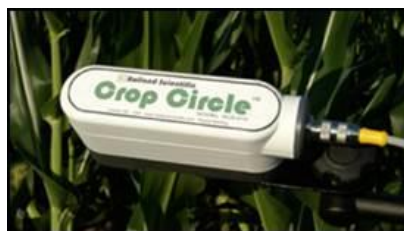
Figure 11-26. A crop circle reflectance sensor
