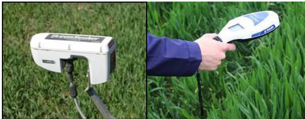
Figure 11-28. A Greenseeker reflectance sensor and a Greenseeker hand held sensor
