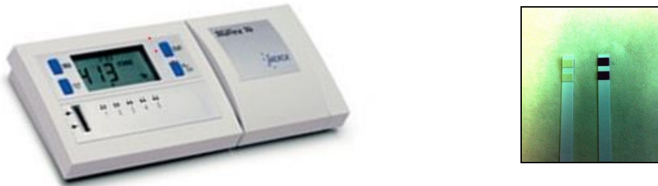
Figure 11-34. Colourimetry-based rapid analysis device and test strips
