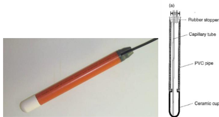
Figure 11-9. Soil solution suction sampler
