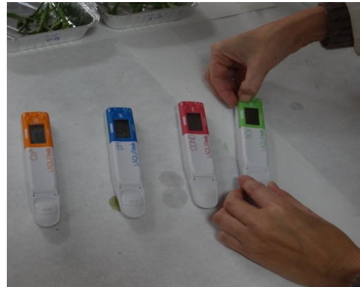
Figure 11-32. Individual selective ion-meters LaquaTwin
