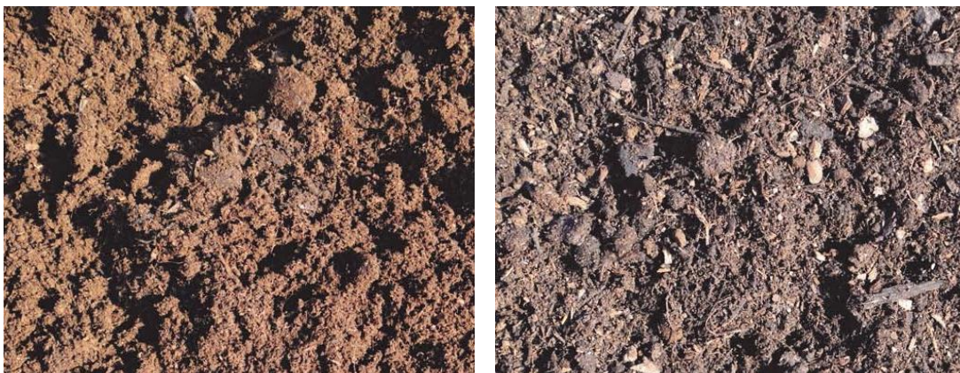
Figure 9-6. Substrate with peat (left) and with peat and compost (right)
