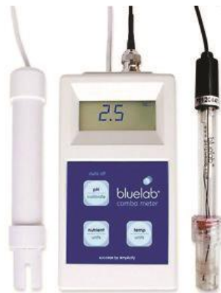
Figure 11-17. EC meter for use in water ( http://www.hydroponics.com.au )
